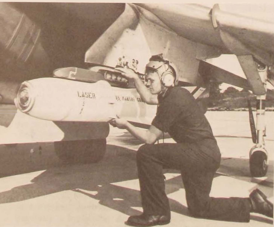
Air-launched cruise missiles (above, on a B-52G) have extended the service life of the aging aircraft and provided a new dimension in employing strategic air power, stand-off attack capability. . . The AGM-65E Laser Maverick (left), here mated to a Marine Corps AV-8B, provides Marine and Air Force ground support aircraft with precise tank-killing capability. . . The AIM-7, shown being fired from an F-15 (facing page), gives U.S. air superiority fighters the high-tech edge.
